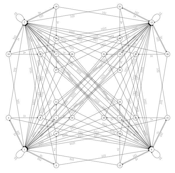
FIGURE 3. Transducer automaton for calculating a minimial joint expansion from the binary expansion.
